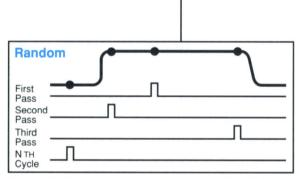
Figure 2. Random-equivalent time sampling digitally reconstructs a waveform using several trigger events.
