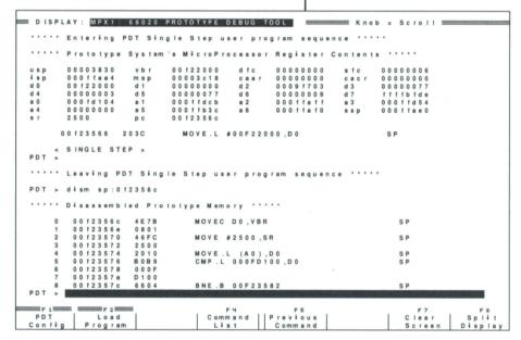
In Single Step mode, the instruction is displayed along with the register contents. This is just one of the emulator commands available on the PRISM Logic Analyzer.
