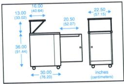
This handsome rackmount workstation provides up to 26 in of rack space, 24 1/2 in with keyboard platform.\*1 The optional side shelf attaches to the extrusion, is easily removable, and can be mounted on either side. (The side shelf is rated at 40 lbs. and measures 16 in x 22 1/2 in.) The K636 cart breathes from the sides and back eliminating any vacuum-cleaner-effect.
