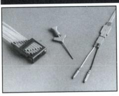
The 100-Channel and 25-Channel probe sets for the 92A96/A96D are based on multiple 8-channel probes, shown above, left. Notice the grouping clip that surrounds the individual podlets. Also shown is a SMT KlipChip $^{TM}$  (206-0364-00), clock probe & clock leadset (020-1888-00, pkg. 12).
