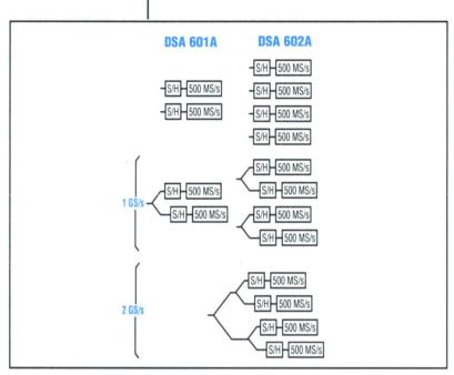
Figure 2. Digitizer interleaving allows for 1 GS/s maximum sample rate in the DSA 601A and 2 GS/s in the DSA 602A.
