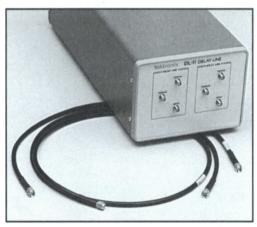
The DL-11 Delay Line contains two delay lines each with 47.5 ns delay. The DL-11 is used for showing the triggering event of a signal displayed on an 11801A or a CSA 803.
