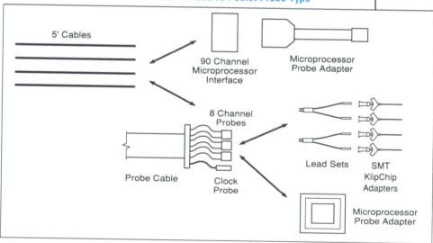
100 Channel Probe Set - Order 010-0492-00 Includes: 96 data (organized as twelve 8-channel probes) & 4 clock probes. Does not include leadsets or KlipChips.
