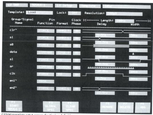
LV500 template setup screen for timing definition.
