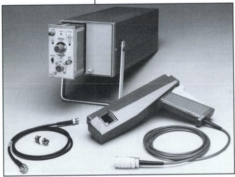
AM503S Current Probe System, Option 03 (A6303 Probe)
