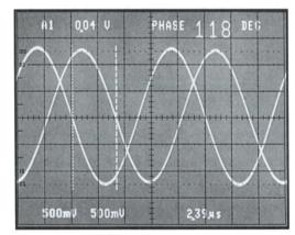
Measure phase shift in degrees or percent. The continuously-calibrated variable sec/div control sets one cycle (360° or 100%) to five horizontal divisions. The time cursors make phase and percentage measurements directly.
