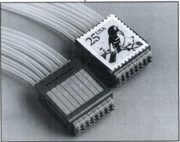
The 92A96 provides the accessibilty needed to observe the many signals of your most complex designs with 8-channel probes the size of the smallest US postage stamp.
