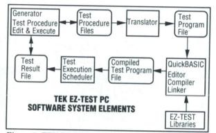
Figure 2. TEK EZ-TEST PC Software System
