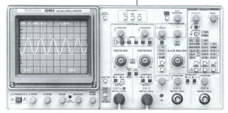
2245A: Ideal for troubleshooting, general repair, and design where basic measurements are often needed. Time and voltage cursors make short work of signal time and amplitude analysis.
