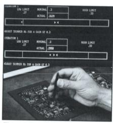
Figure 1. The adjustment step acquires measurements and displays them on screen relative to nominal and upper and lower test limits, simplifying UUT adjustment procedures.
