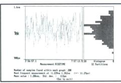
Measurement features of the 11000 Series DSOs are available through the menus and are supported by measurement logging, statistics, and screen graphics.
