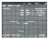
The Option 05 Video Measurement System allows selection of individual lines and fields. Here, Line 49 from Field 1 is selected.
