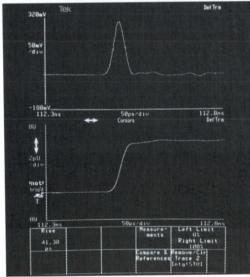
High-Speed Optical Impulse and Calculated Optical Step Response
