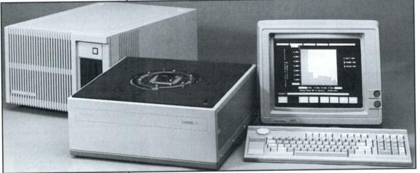
The LV500 provides up to 16 clock sources (timing generators). Each of the data channels is assigned to one of the 16 clocks. Events on any data channel are programmed to occur on either of the clock edges. As with large testers, the test cycle length may be changed from one cycle to the next.
