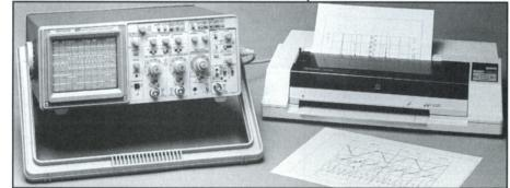
For convenient documentation you can link the 2211 or 2201 to a 4-color plotter such as the HC100, to brint the waveform record.
