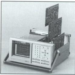
Both the 1230DSM and 1230E1 cards install easily allowing you to reconfigure your instrument in less than five minutes.
