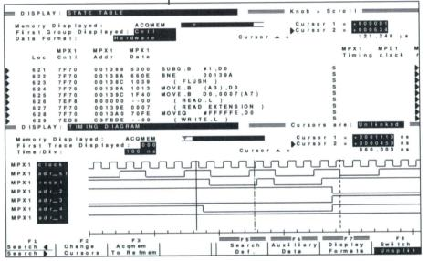
PRISM's split screen display can display both state and timing at the same time. The "link curser" option links the two displays together so as one display scrolls, the second display stays in sync.
