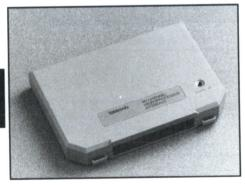
The 90-Channel Microprocessor Interface allows existing 92A60/A60D or 92A90/ A90D microprocessor probe adapters to work with the 92A96/A96D. Order 010-0508-00.
