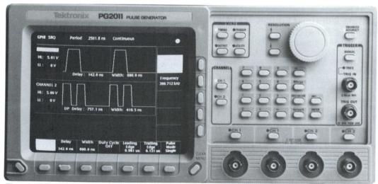
The new PG2010 family has representative waveform display, important pulse parameters, and softkey menus all on the crt.
