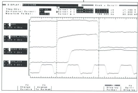
Multiple waveforms can be freely moved and sized on screen. Not only can you see the time relationship between these waveforms, but the quality of the signals as well.
