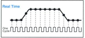
Figure 1. Real-time sampling captures a complete waveform with a single trigger event.
