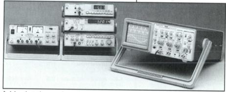
Lab bench stations can be configured to your needs. Our stackable triple-output power supply, digital multimeter, 100 MHz frequency counter and 2 MHz function generator (see pages 246 and 248) join a 50 MHz dual-trace oscilloscope (page 106) as a popular setup for basic lab stations.
