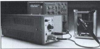
Tek's versatile AM 503S Current Probe System lets you measure and display both ac and dc current waveforms from dc to 50 MHz. See page 325 for details.
