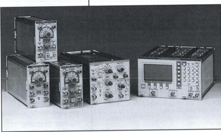
PG 501, PG 502, PG 503, PG 508 and PG 5110 Pulse Generators.
