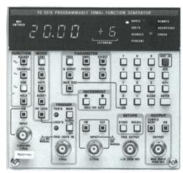
**Trigger Output** – 0  $\pm$ 100 mV to  $\geq$  2 V from 50  $\Omega$  into an open circuit.
