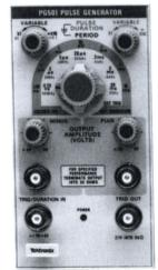
The PG 501 is a 50 MHz Pulse Generator featuring simultaneous plus and minus outputs, a wide range of pulseperiod durations and duty factors, trigger output, and external trigger/duration input. Its performance and ease of operation make it well-suited to basic digital and analog applications.
