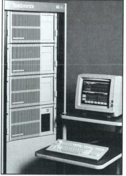
Up to three expansion mainframes can be connected to the DAS9219 or DAS9220 expanding the system to 28 instrument card slots. For automated test (ATE) applications. the DAS9200 can be setup and controlled via RS-232 or GPIB interfaces.
