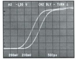
Adjustable delay increases accuracy. A frontpanel knob adjusts the Channel 2 delay to exactly match the Channel 1 delay from the probe tip.
