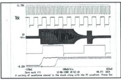
Multiple waveforms can be acquired and displayed on the PC screen and output to a plotter or dot-matrix printer.
