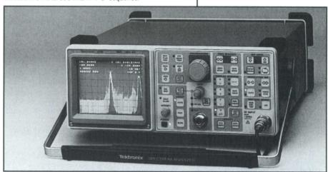
Freq. Span/Div Range - 2712 (2710 w/opt. 01): 180 MHz to 1 kHz. 2710: 180 MHz to 10 kHz selected in 1-2-5 sequence or 2 significant digits via menu.
