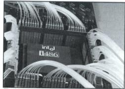
The high-bandwidth probes and advanced 100 MHz clocking state machine of the 92A96 allow the 92A96 to interfaced to virtually any processor or bus without a complex, bulky hardware interface.
