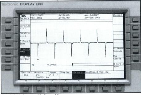
Front Panel close-up with Cursor Measurements
