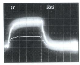
A pulse train with a low level pulse on the 7104, with one thousand times the brightness of conventional oscilloscopes. The researcher can view the pulse directly and take pictures with ease.
