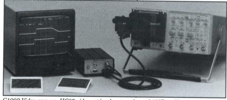
C1002 Video camera, HC02 video copier documenting a 2467B oscilloscope's display using a DX02 power supply.
