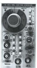
gating are provided with a variable phase control to permit up to ±90° of phase shift for generating haver-sines, sine pulses, and haver triangles. A step attenuator provides 60 dB of output signal attenuation in 20 dB steps with an additional 20 dB of variable attenuation. Variable symmetry from 5% to 95% provides ramps and pulses. Pulse rise time is ≤ 25 ns. Audio sine-wave distortion is  $\leq 0.25$  and audio amplitude flatness is within 0.1 dB.
