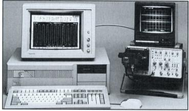
The Digitizing Camera System consists of a C1002 Video Camera, Frame Store Board inside the PC, DCS software, and cables. The system shown includes the DCS, TEK 2467B scope under GPIB control from the DCS software, and a DX05 video monitor.
