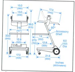
The K212 base is made of thermoset polyester; the column and trays, high-strength aluminum. The base and trays are Tek Blue; column and yoke, silver grey
