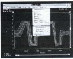
Create the reference memory template waveform for pass/fail testing on 2400 series oscilloscopes.
