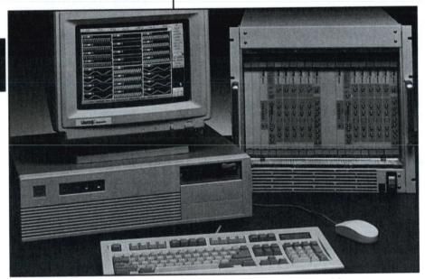
Simultaneous display of 24 waveforms using the AZIM1 Interactive Measurement Software.
