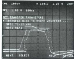
DSO Utility Software includes routines to create waveshape templates, compare live signals against the templates for automatic pass/fail tests, and archive waveform and measurement
