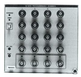
Voltage Standing Wave Ratio (VSWR) — Any 4 Channel Group: 1.25:1 at 100 MHz, increasing to 1.8:1 at 350 MHz. Any Other Combination: 1.5:1 at 100 MHz. 2:1 at 225 MHz.
