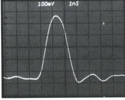
View of a single clocking pulse of 0.8 ns rise and 2 ns pulse width.
