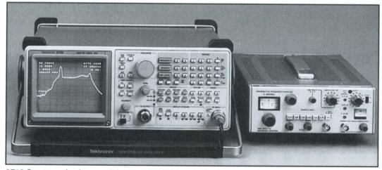
2712 Spectrum Analyzer and the 1405 TV Sideband Adapter
