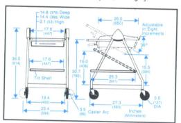
These sturdy, portable carts are ideal for manufacturing, research and design environments. The tiltable middle tray on the K217S is rack width to accommodate additional instruments.
