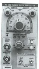
pulse generator useable in either the TM 500 or TM 5000 series mainframes. It is identical to the PG 502 except for output which is now differential; the risetime is faster, and the amplitude range is 2.5 V within a ±2.5 V window. The fast risetime makes the PG 503 ideal for testing the new high-speed ECL and GaAs logic families.
