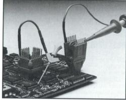
PLCC Quad Clip (left) and SOIC Clip (right).
